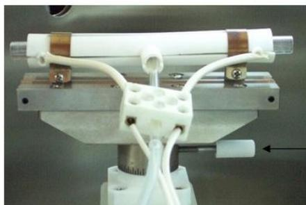
Fastening knob of rotation angle adjustment for the burner
