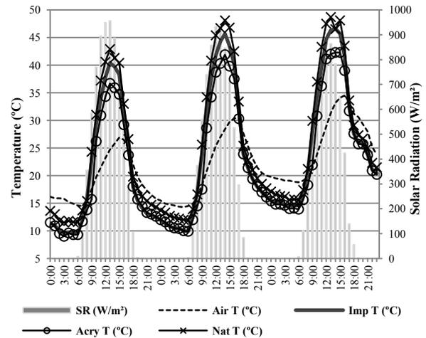
Figure 4: Reflective cooling on roofing and solar radiation on 3 consecutive days on dryer period.
