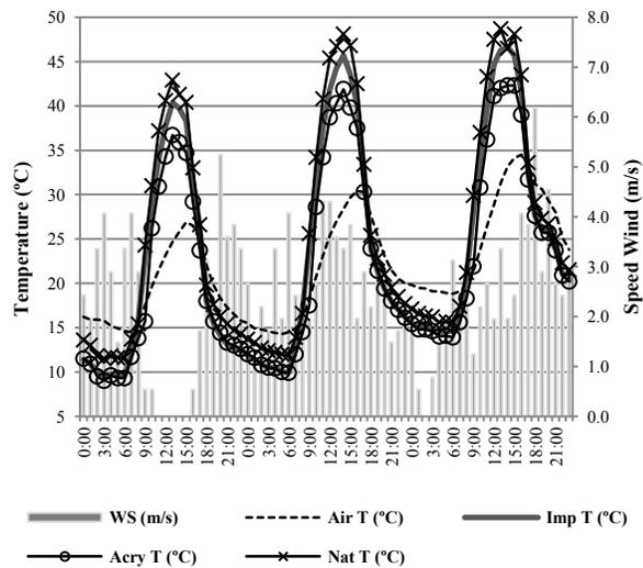
Figure 5: Reflective cooling on roofing and wind speed during 3 consecutive days on dryer period.
