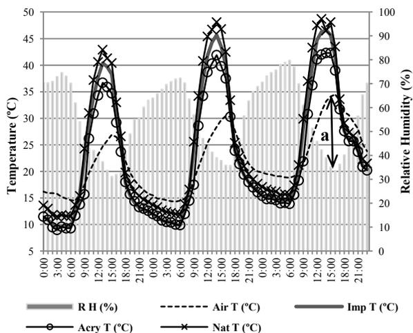
Figure 6: Reflective cooling on roofing and relative humidity air during 3 consecutive days on dryer period.
